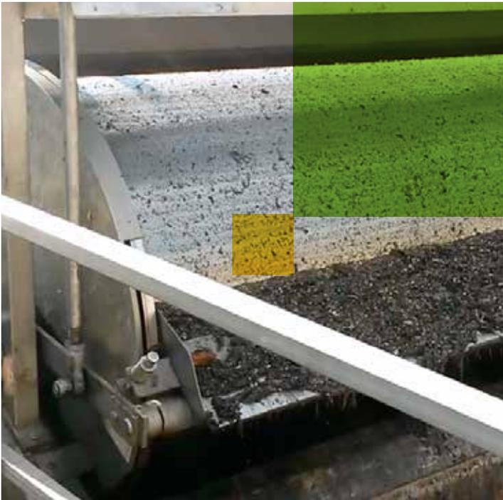
The Sliding Blade System is a special equipment of the IDRASCREEN®, outcome of continuous research to solve those difficult cases where the effluents contain a high amount of fibres. These fine particles can become wedged under the doctor blade. The solution to this problem is the sliding blade device.
