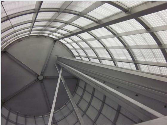
Hydrotech's patented filter panels improve the hydraulic capacity and offers better lifting properties. The drum is constructed in sections, each with up to 5 filter panels depending on diameter. This makes it easy to design a solution according to your specific requirements.
